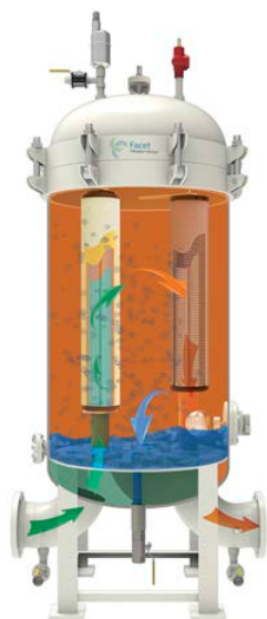
Vertical Two-Stage Coalescer Separator Flow Diagram
