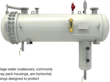
Facet HP Series single-stage water coalescers, commonly referred to as repack or hay pack housings, are horizontal, cylindrically shaped housings designed to protect filtration systems from gross amounts of water and solid contaminants. Facet recommends using their wafer style repack coalescers since they allow the first two sections to be replaced when required. The third and successive sections require fewer change outs since they may remain relatively free of solids.
